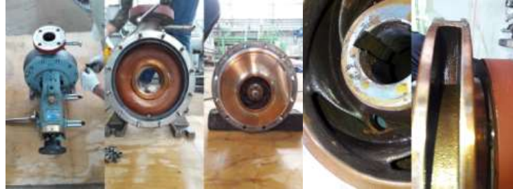
(a) casing (b) impeller Fig.11 Inspection after pump test
